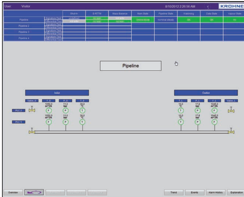
Figure 3-4: Example of pipeline details
