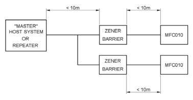
Each MFC010 <u>MUST</u> have its own dedicated barrier interface; they <u>MUST NOT</u> be connected in parallel on the hazardous area side of the system.
