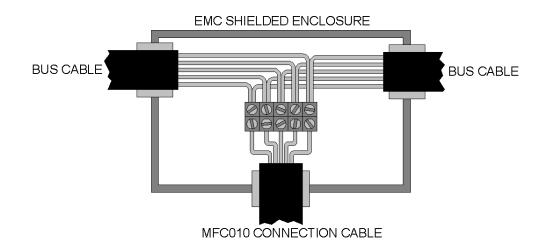
If the Bus does not provide a suitable power supply for the MFC010, a separate suitable power supply connection should be made at this point.
