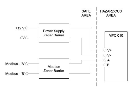
The Zener barrier devices must be installed in an E MI shielded enclosure and the cable screen(s) kept intact right up to the barrier terminals as far as is practical. The cable screen(s) should be terminated to the enclosure, chassis Earth connection, and kept <u>SEPARATE</u> from t he intrinsically s afe E arth connections of the Barrier devices. The user <u>MUST</u> adhere to the barrier manufacturer's instructions for connecting the intrinsically safe Earth connection to the barrier devices.
